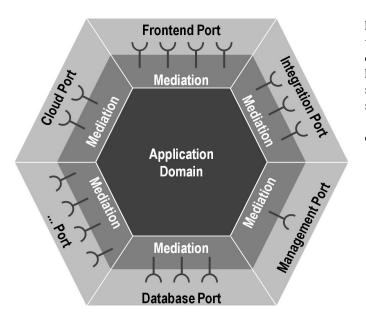
Figure 2. Hexagonal Architecture
