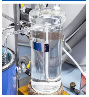
▲ Vapor pressure measurements: The transpiration method is one of the four methods that we use to determine vapor pressures in every desired temperature and pressure range
