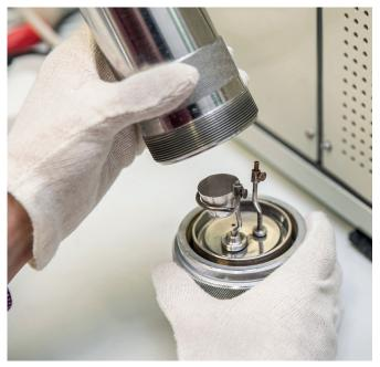
▲ High precision combustion calorimetry: With our special combustion calorimeter, we can determine combustion enthalpies and enthalpies of formation with a precision that is up to 10 times higher than the results from commercial devices
