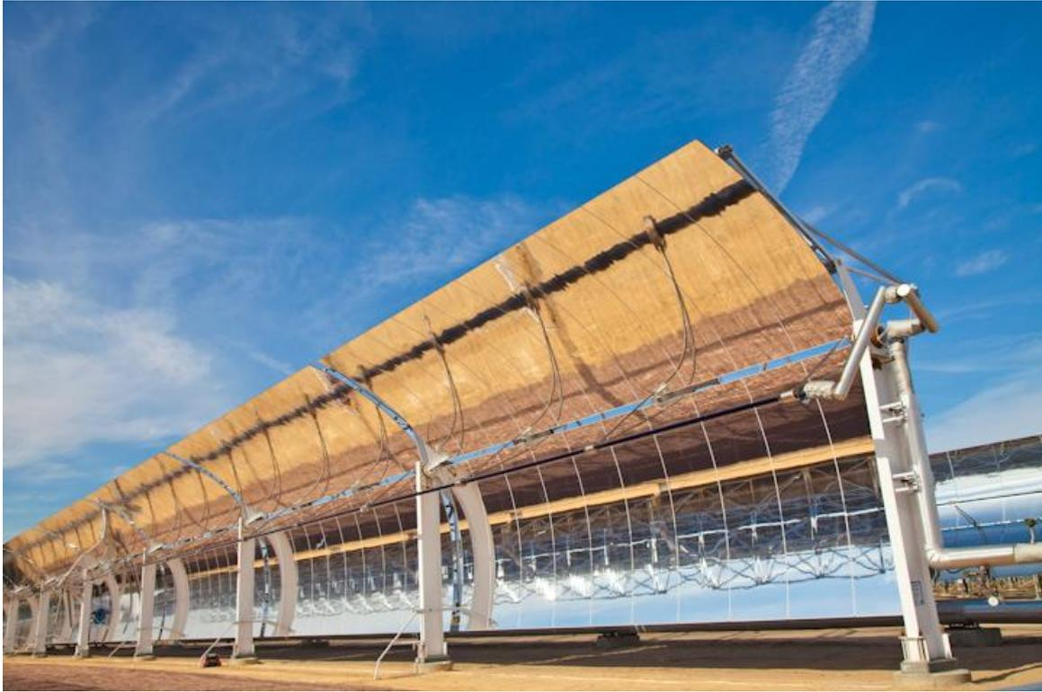
Figure 2. Parabolic trough collector [9]
