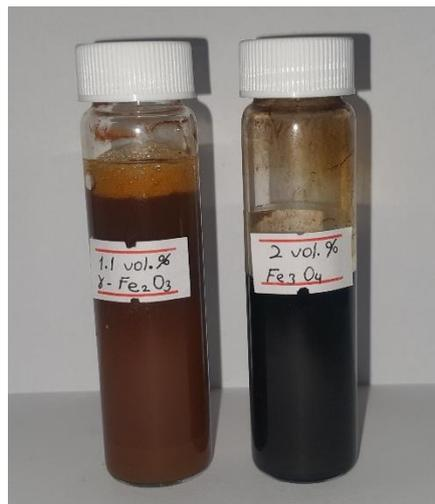
**Figure 1. ( $\gamma\text{-Fe}_2\text{O}_3$ ) - water and  $\text{Fe}_3\text{O}_4$  - water magnetic nanofluids with 1.1% and 2% volume concentrations, respectively**
