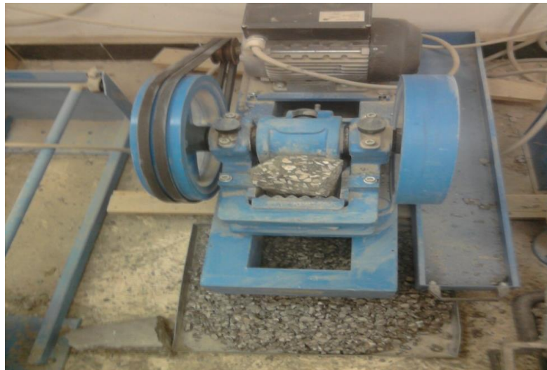
Figure 1 : Concrete fragment crushed used to produce recycle aggregates
