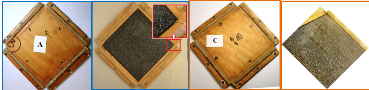
Fig. 8. Typical failure of plywood specimens in sample type of A and C; the initial state and destruction
