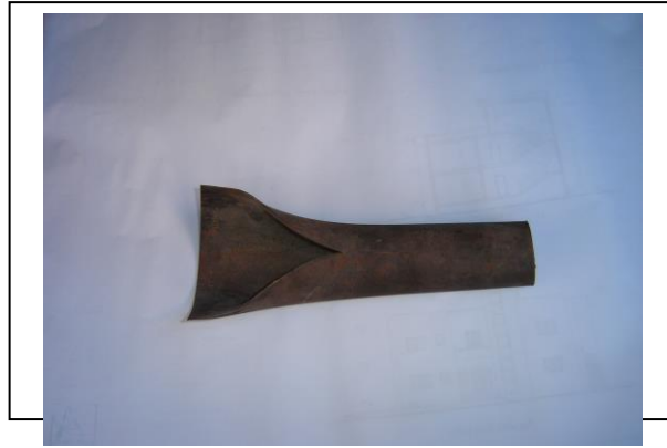
Figure(2) Close-up view of ruptures superheater tube
